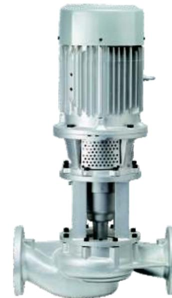
The NTT, NBT and NIT product series are ideal for moving mineral-based thermal oils. Their mechanical seals are located behind a heat barrier, where they are protected from high temperatures. The result is that simple standard gaskets (antimony-carbon/SiC) have a very long service life when used in the pumps. All three types are also available as two-stage versions with the same external dimensions, making them ideal for small flow rates with high delivery head.
