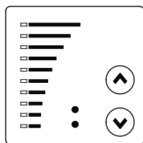
Fig. 21 Control panel of a CME pump
