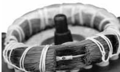
Fig. 42 PTC sensor incorporated in windings
