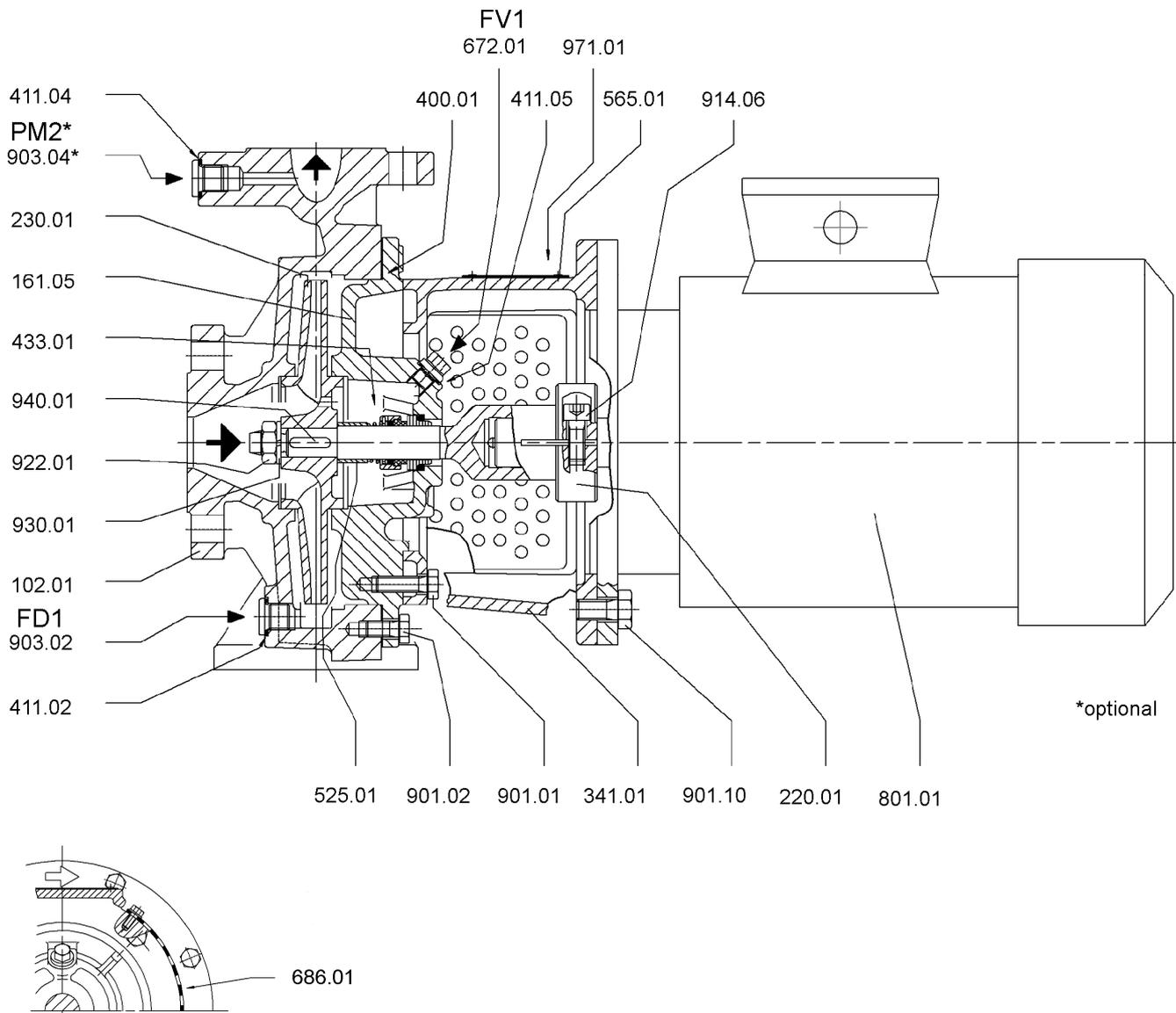
Fixing of guard plate to the drive lantern.
