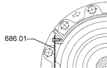
Fixing of guard plate to the drive lantern.
