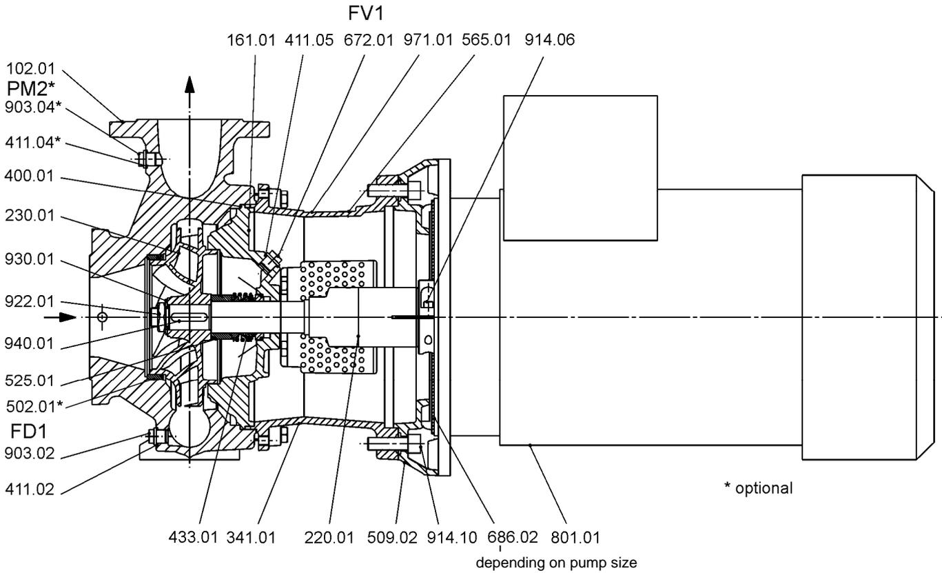
Uncooled, unbalanced mechanical seal
