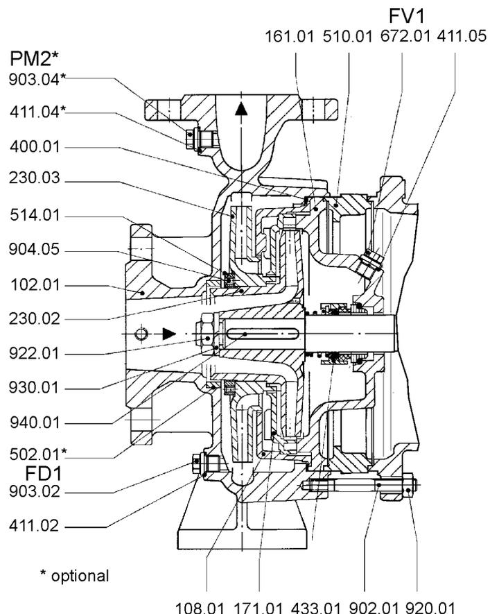
Two-stage sizes with shaft diameter 30 at the shaft seal, uncooled, unbalanced mechanical seals
