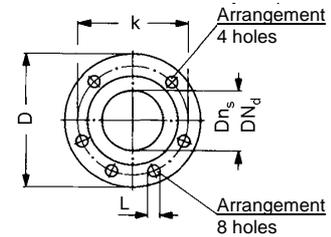
Connections at sizes 25-200 and 2/25-200: FD1= G 1/2; FF1 at sizes 20-160, 25-200 and 2/25-200 not existent.
