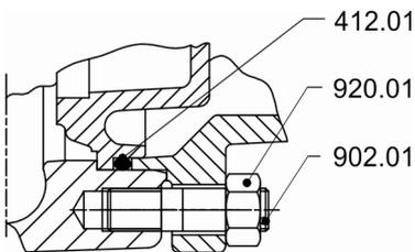
Sizes with shaft diameters 24 at the shaft seal
