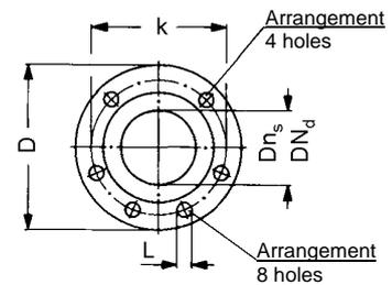
Tolerances of companion dimensions acc. to DIN EN 735
