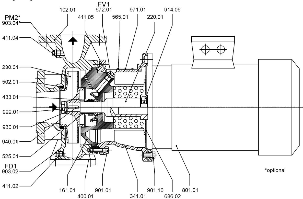
Uncooled, unbalanced mechanical seal
