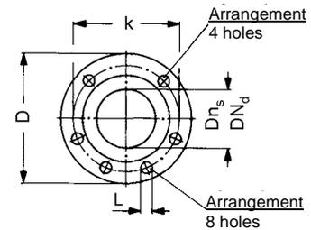
Connections at sizes 25-200 and 2/25-200: FD1= G 1/2; FF1 at sizes 20-160, 25-200 and 2/25-200 not existent.
