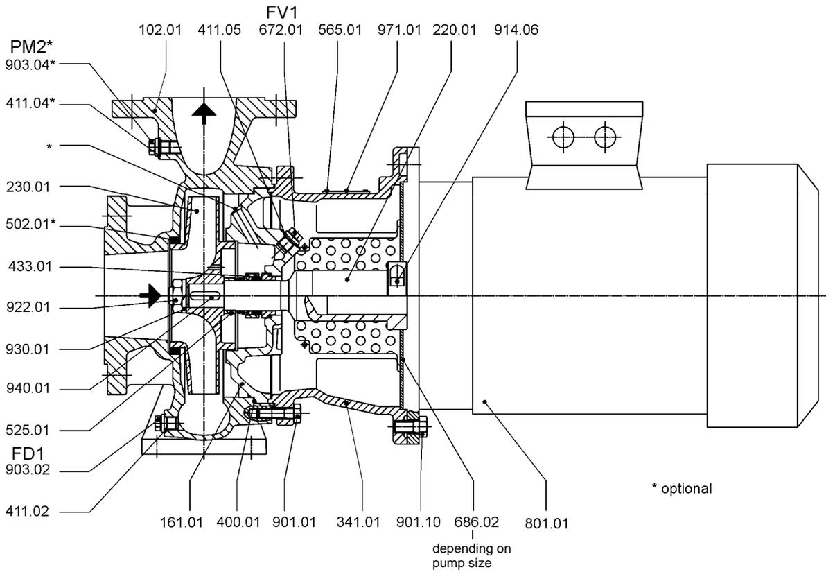
Uncooled, unbalanced mechanical seal
