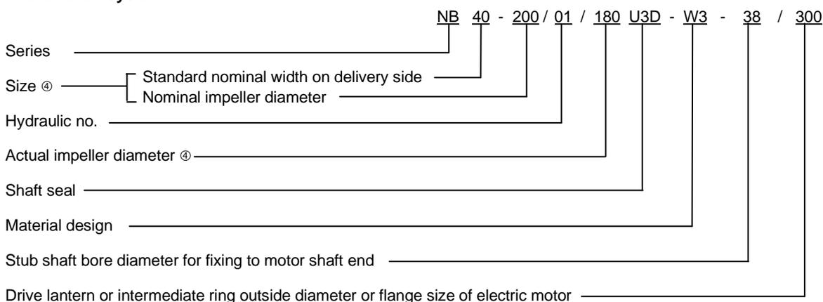
④ The actual impeller diameter of two-stage sizes relates to the second stage. The number of stages is placed in front of the nominal width of the outlet branch, e.g. 2/40-200/...
