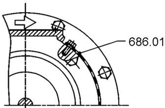
Fixing of guard plate to the drive lantern.
