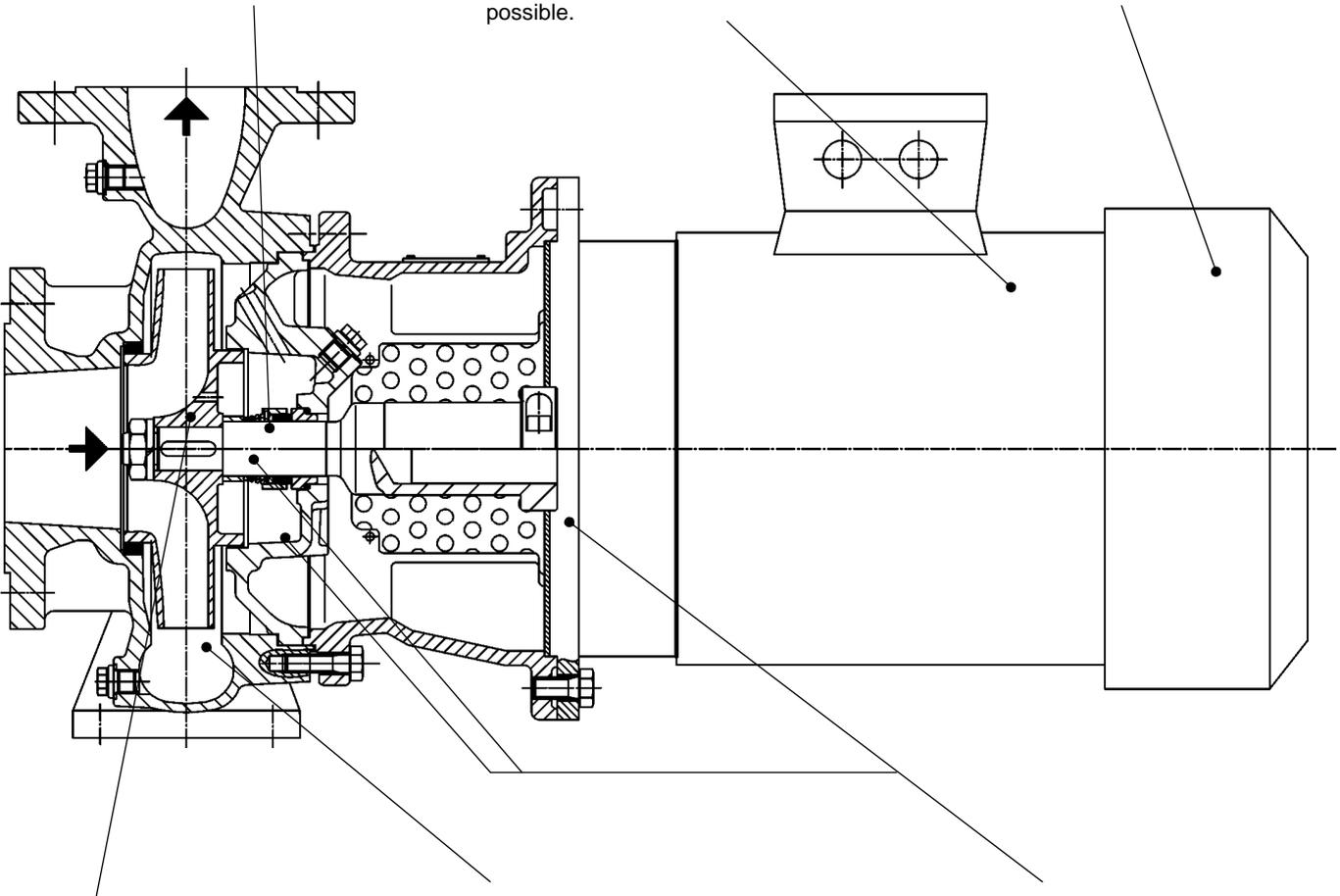
**Negligible axial thrust** by fine adaption of the balancing holes.
