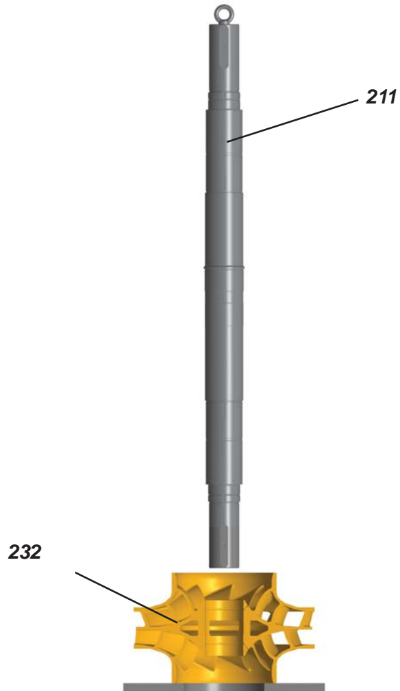
Fig. 8-17 Installation of the impeller
