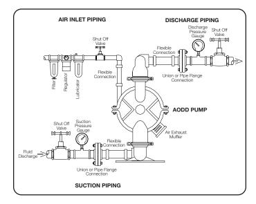
Suction pipe size should be at least the same diameter as the inlet connection size, even larger if highly viscous fluid is to be pumped. If suction hose is used, it must be of a non-collapsible reinforced type. Discharge piping should be of at least the same diameter as the discharge connection. It is critical,
