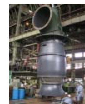
Vertical mixed-flow pump with variable pitch vane
