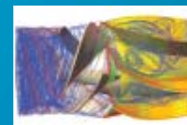
Internal flow visualization of mixed-flow pump
